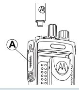
3 Secure the connector cover to the radio by turning the thumbscrew clockwise.
