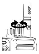
Once the required zone is displayed (if you have multiple zones in your radio), turn the programmed Channel Selector Knob to select the call type.
