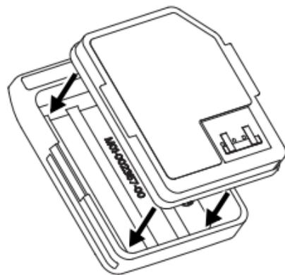
4. Replace the alkaline battery tray cover.
